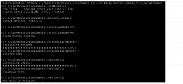
Figure 3: Console display after successful MCS download with FMP.
