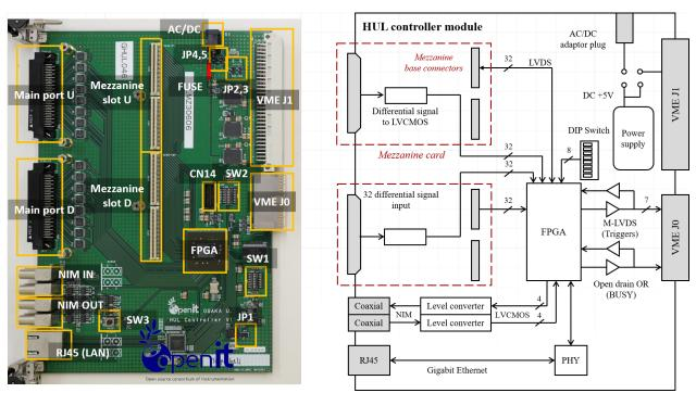
Figure 1: Photo and block diagram of HUL controller.
