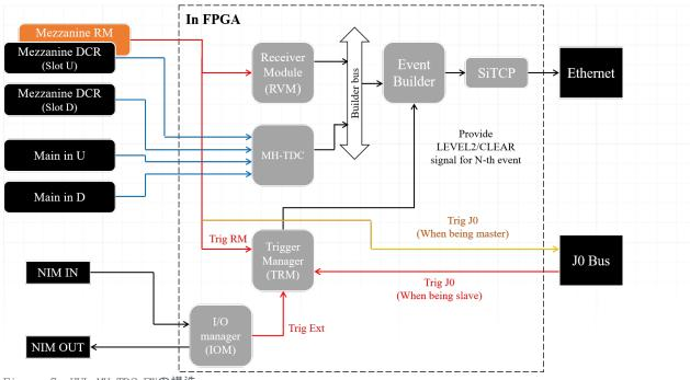
Figure 7: HUL MH-TDC FWの構造。
