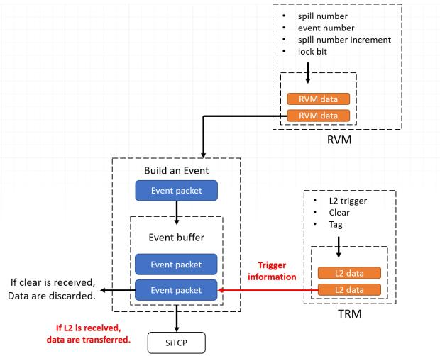
Figure 4: DAQ data flow of HUL RM firmware
