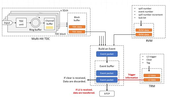
Figure 8: DAQ data flow of HUL MH-TDC firmware
