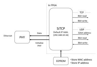
Figure 1: SiTCP block diagram
