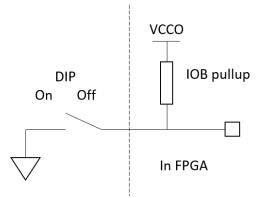
Figure 1: Circuit diagram of DIP SW
