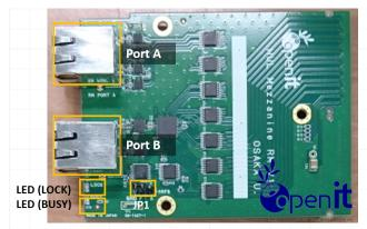
Figure 5: HUL receiver module (HRM)
