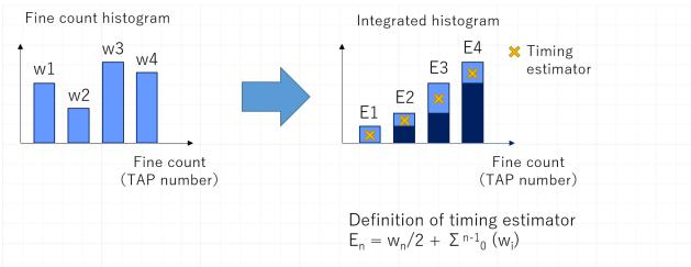
Figure 11: Procedure to generate estimators from fine count histogram.
