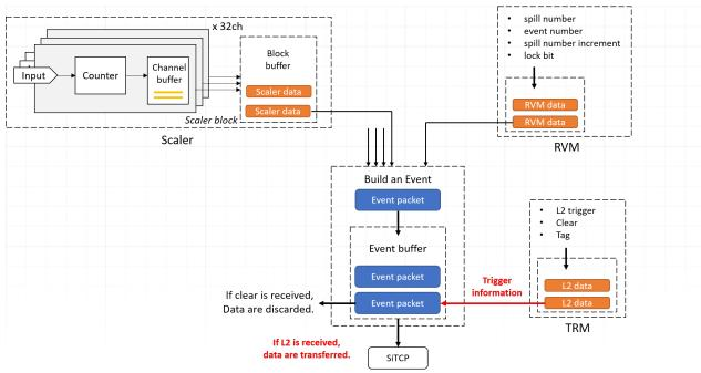
Figure 6: DAQ data path of HUL Scaler firmware
