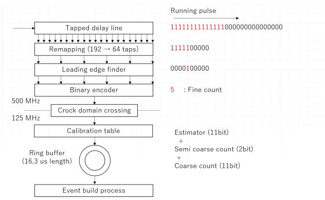
Figure 13: Block diagram of HR-TDC
