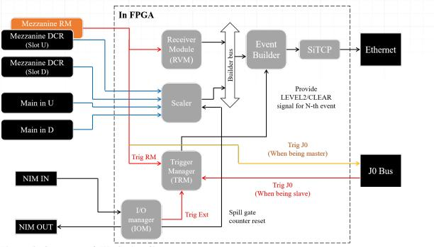
Figure 5: Structure of HUL Scaler firmware
