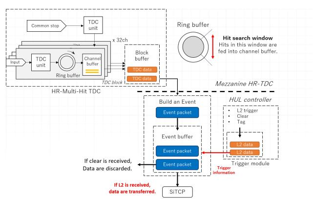
Figure 14: Data flow block diagram of Mezzanine HR-TDC and HUL HR-TDC BASE
