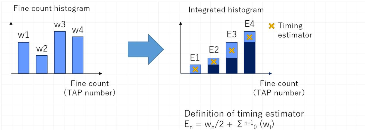
Figure 11: Procedure to generate estimators from fine count histogram.
