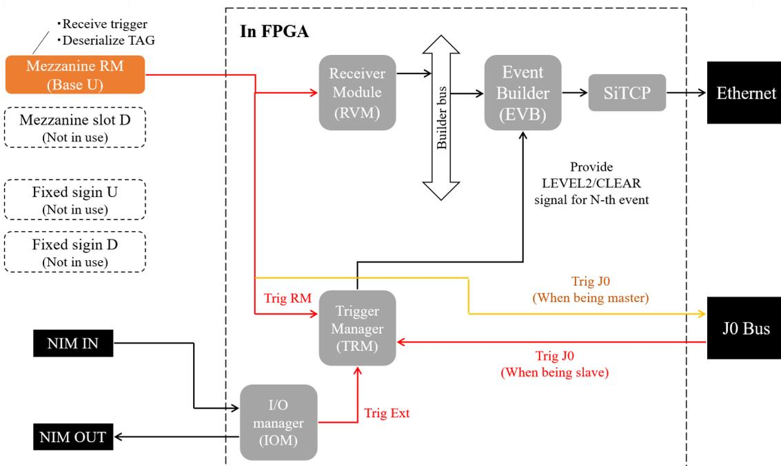
Figure 2: HUL RM firmware block diagram
