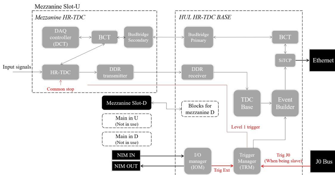
Figure 9: Block diagram of HUL HR-TDC firmware
