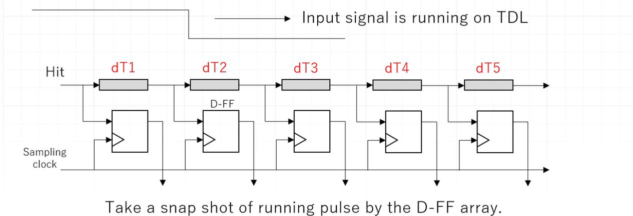
Figure 10: Schematics of Tapped-delay-line
