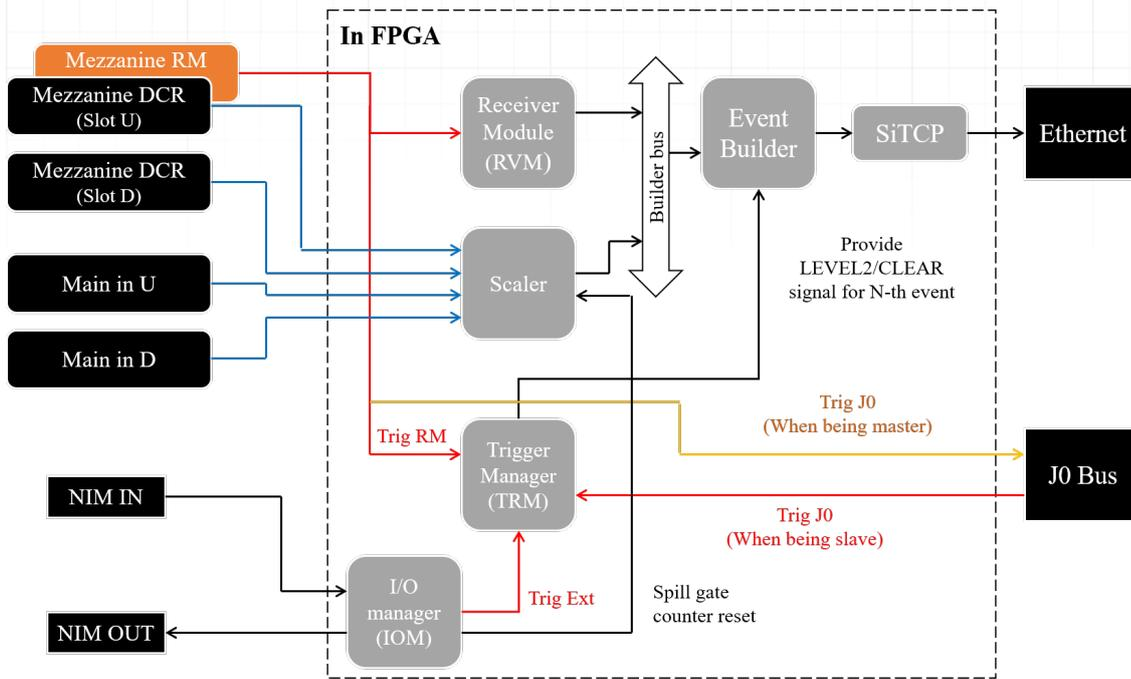
Figure 5: Structure of HUL Scaler firmware
