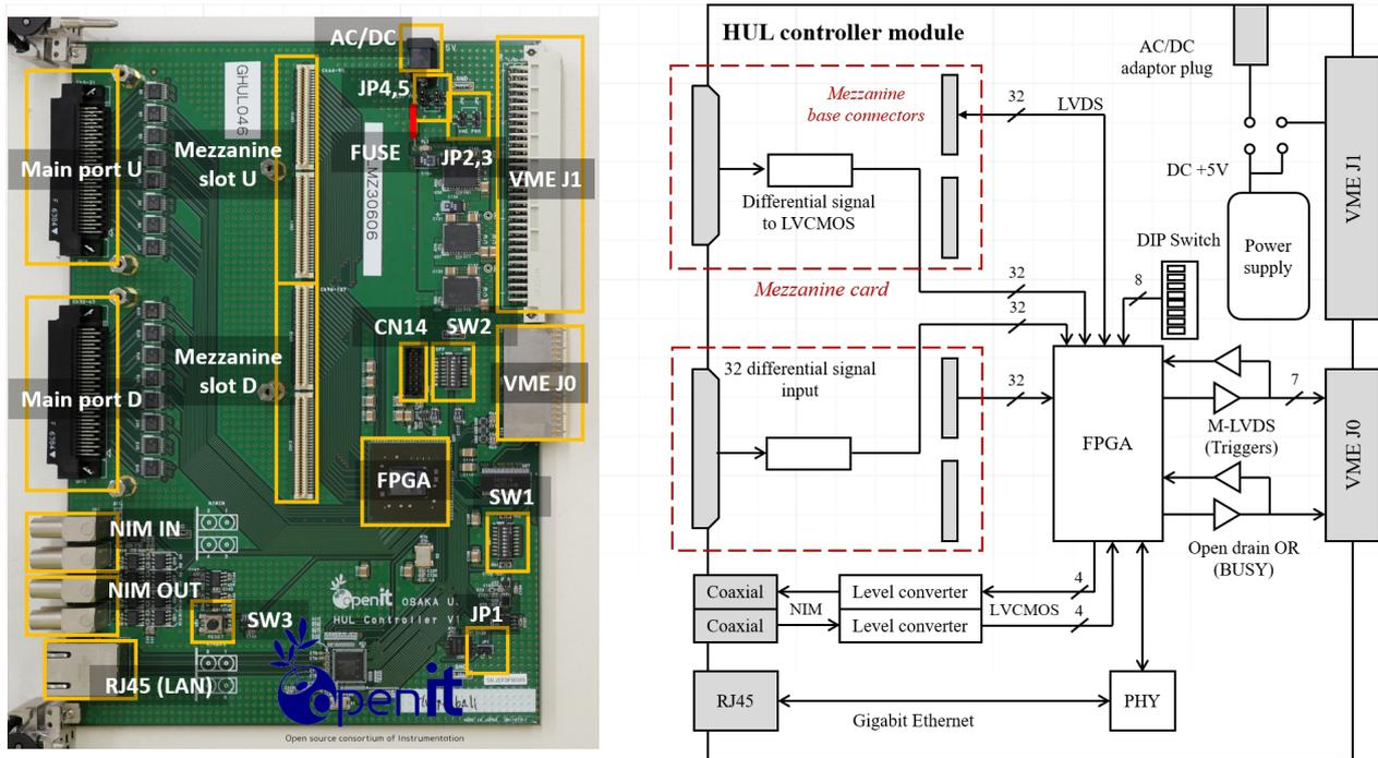
Figure 1: Photo and block diagram of HUL controller.
