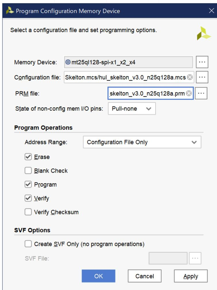
Figure 2: Configuration Memory Device
