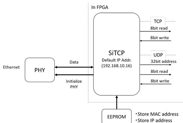
Figure 1: SiTCP block diagram
