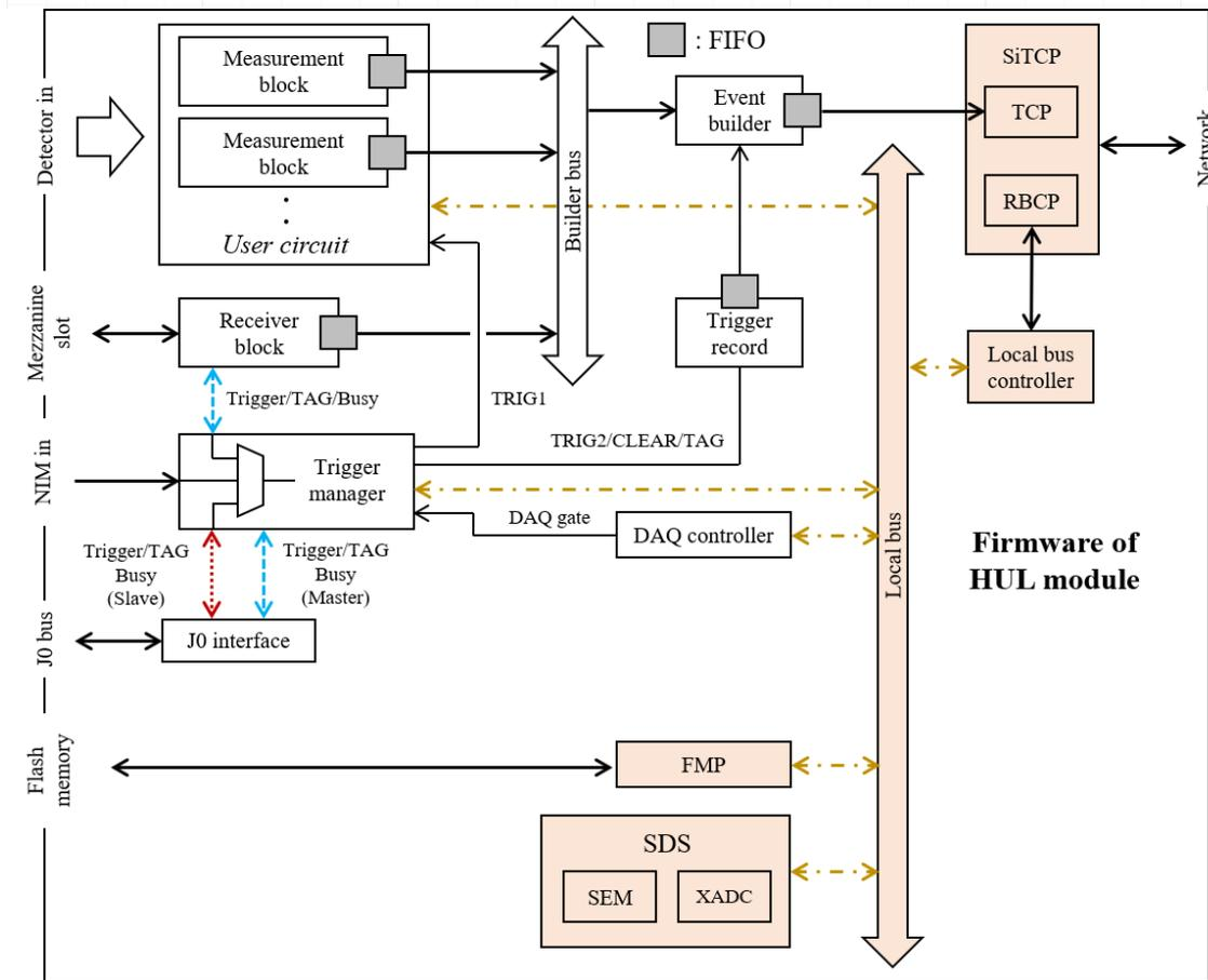
Figure 1: Block diagram of data-acquisition-type firmware
