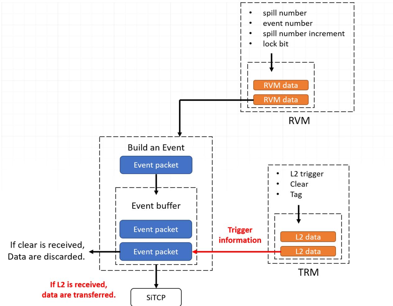
Figure 4: DAQ data flow of HUL RM firmware
