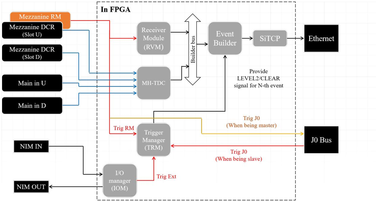
Figure 7: HUL MH-TDC FWの構造。
