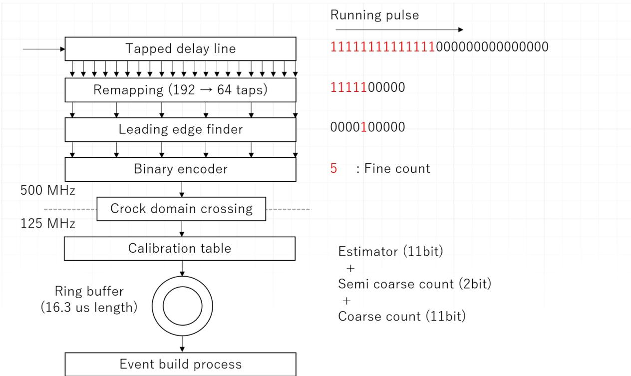
Figure 13: Block diagram of HR-TDC
