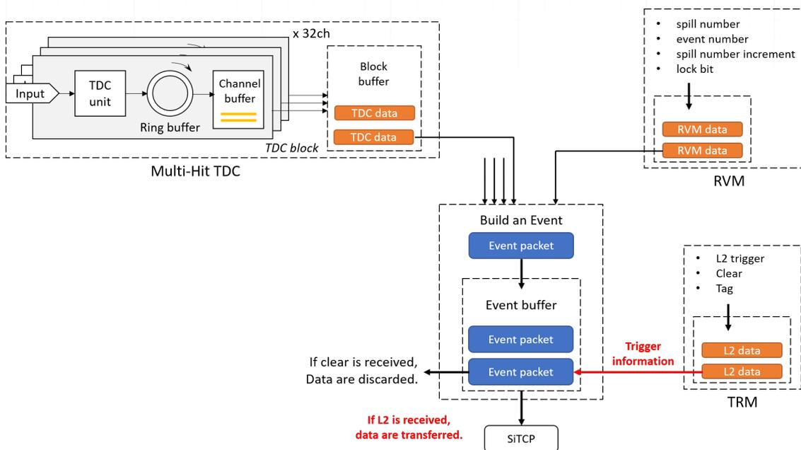
Figure 8: DAQ data flow of HUL MH-TDC firmware
