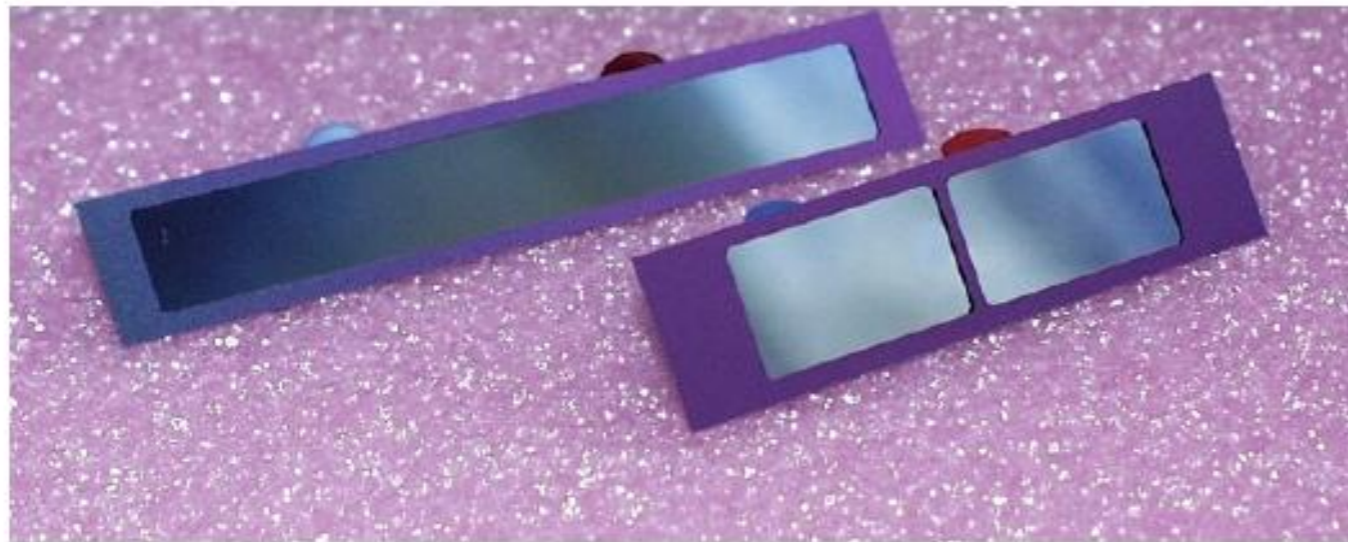
first 'dummy' samples: 50 \mu\text{m} silicon with 350 \mu\text{m} frame
