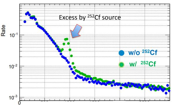
Can see clear excess due to neutron capture on Gd.
