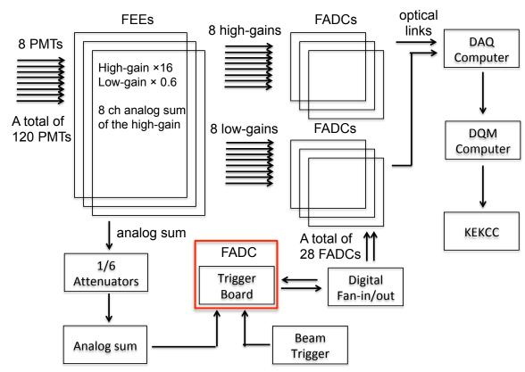
Using special amps with two different gains.
