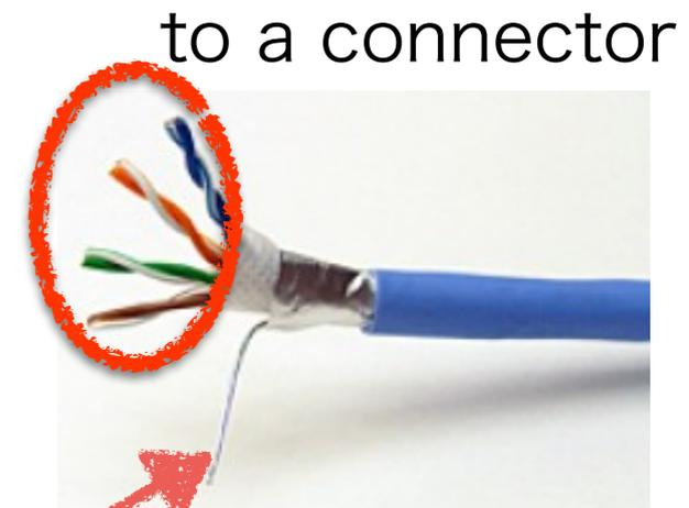
pigtail : to ground/shield case
