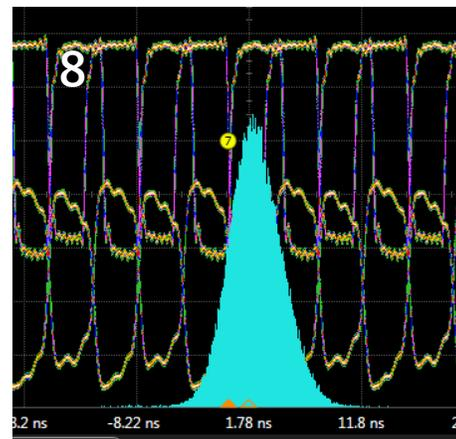
Edge-to-Edge measurement reflects the structure of the main peak of the jitter distribution.
