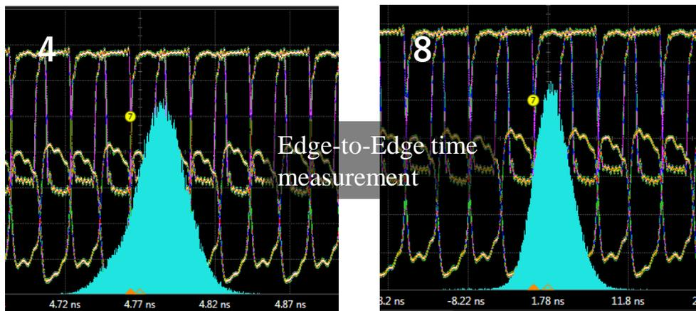
Edge-to-Edge measurement reflects the structure of the main peak of the jitter distribution.
