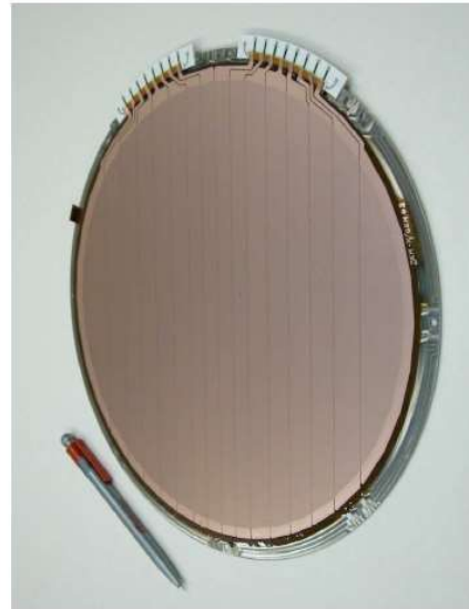
ESA-INTEGRAL Mission Prototype GEM for JEM-X (25 cm \emptyset ):
