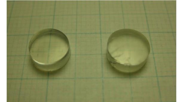
Photograph of 40 wt% (left) and 60 wt% (right) Hf-PLSs, approximately 8 mm in diameter and 3 mm in thickness.
