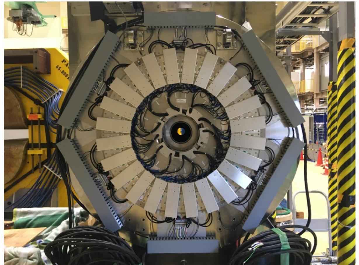
CYCLOPS under commissioning Scintillating fiber+SiPM +ASIC+FPGA+SiTCP, 3008 ch.
