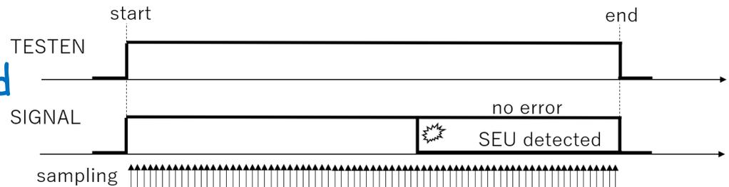
Schematic view of evaluation circuit for SEU
