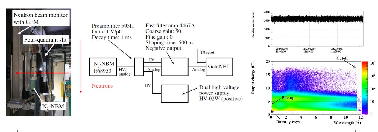
Beam power: 793 kW, T0 chopper: 25 Hz mode,  $L_1$ : 13.76 m, Beam size@nGEM: 3.44 × 3.44 cm<sup>2</sup>
